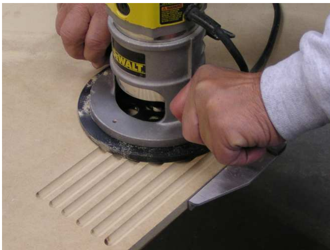
Using Fence to cut flutes
