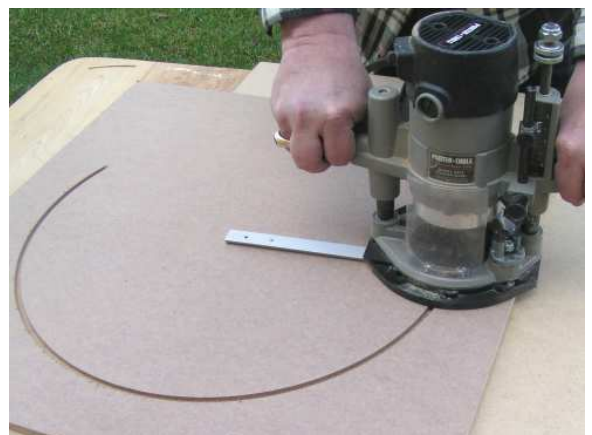
Router Buddy cutting circle
