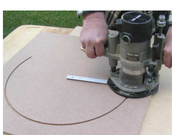
Router Buddy cutting circle
